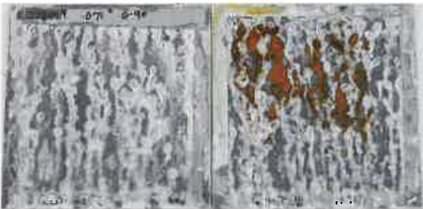
12338019 .071" G90 - 1008 hrs Salt Spray - ASTM B117
