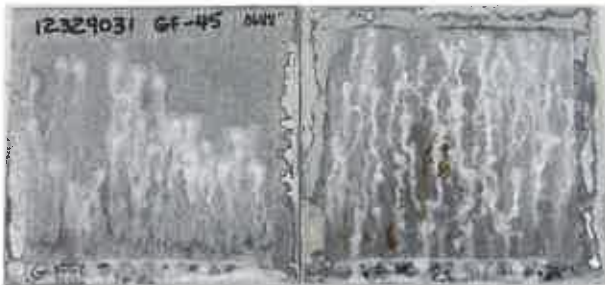
12329031 .0648" GF45 - 1008 hrs Salt Spray - ASTM B117
