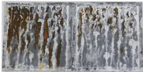
22311056 .0142" G60 - 1008 hrs Salt Spray - ASTM B117
